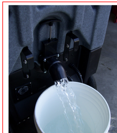
Drain water from Recovery Tank
