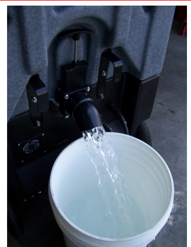
Draining the Recovery Tank
