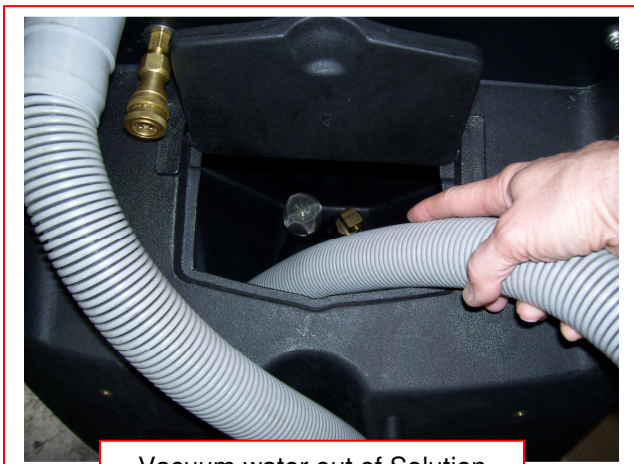
Vacuum water out of Solution Tank
